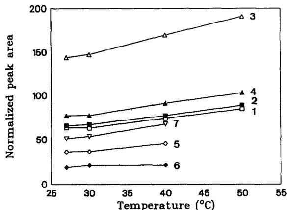
Fig. 4. Relationship between temperature and normalized peak areas of aromatic choline esters. Numbers as in Fig. 1. Other conditions as in Fig. 3.
