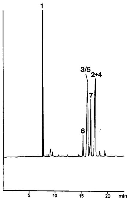
Fig. 2. Electropherogram of the mixture of aromatic choline esters separated by the MECC method (TTAB). Numbers as in Fig. 1. Separation conditions: buffer composition, 30 mM disodium hydrogenphosphate–18 mM disodium tetraborate–50 mM TTAB–5% 2-propanol; temperature, 40°C; voltage, –18 kV; total length of capillary, 760 mm; detection 530 mm from injection end; UV detection at 235 nm. Vacuum injection for 1 s.
