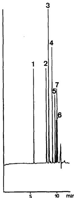
Fig. 5. Electropherogram of the mixture of aromatic choline esters separated by the MECC method (NaCh). Numbers as in Fig. 1. Buffer composition, 100 mM disodium hydrogenphosphate–500 mM taurine–35 mM NaCh–2% 2-propanol. Other separation conditions as in Fig. 3.
